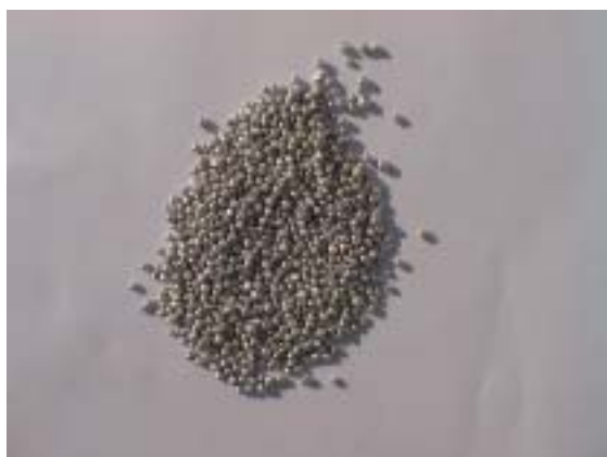
I.-No. 8024 Aluminium granule, round graining 2,0 – 4,0 mm
