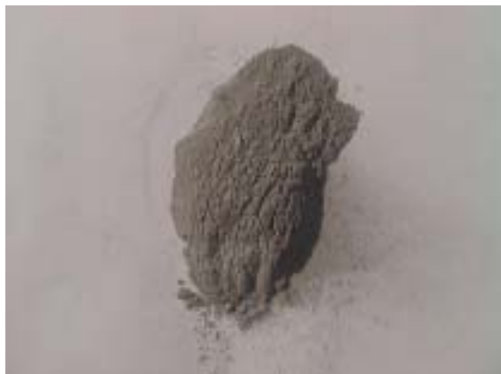
I.-No. 4065 Aluminium particle graining < 65 µm
