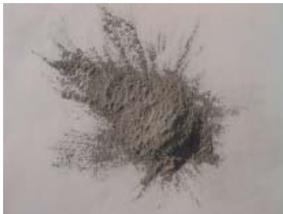
I.-No. 4150 Aluminium particle graining < 150 µm
